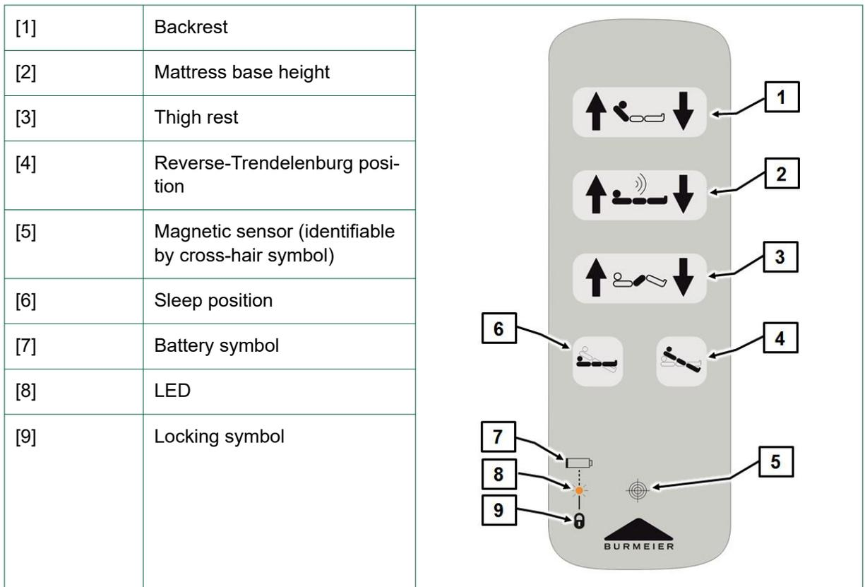
**i** Adjust the mattress base height whenever necessary, but at least once a day, to the uppermost or lowest height. This automatically equalises the two independent adjustment drives and results in a level horizontal mattress base.
