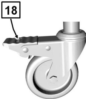
The bed stands on four steerable castors which are all fitted with a locking brake.
