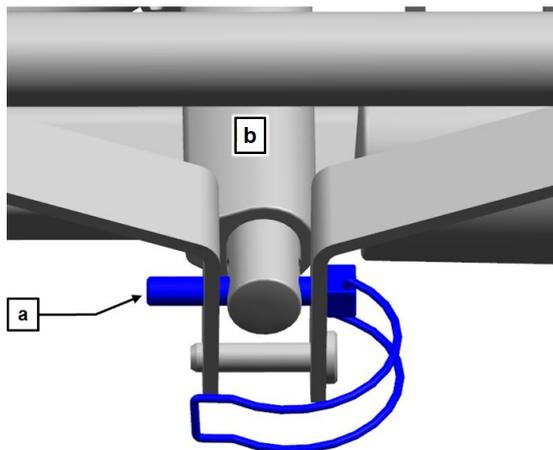
3. The second person now removes the locking pin [a]. To do so, swivel the curved clip away and draw the bolt and pin, together with the clip, out of the backrest motor lifting pipe [b].
