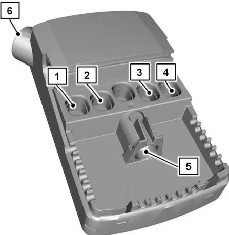
The diagram shows a perspective view of the CA 40 drive system. A power supply connector (6) is located on the left side. On the top surface, there are four circular ports labeled 1, 2, 3, and 4. On the bottom surface, there is a rectangular connector labeled 5.
