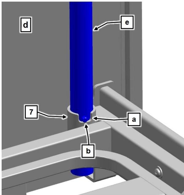
There are two round lifting pole adapter sleeves at each corner of the head end [d] of the mattress base frame. There is a notch [a] on the top surface of the lifting pole adapter sleeve that, together with the pin [b], restricts the slewing range [c] of the patient lifting pole. The lifting pole should be fitted to the side of the bed that the resident uses to get in and out of bed.
