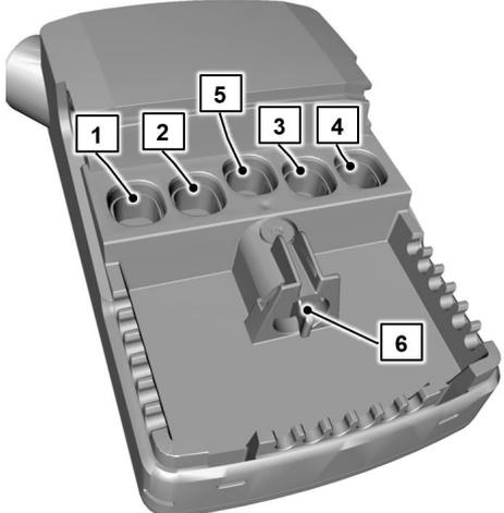
**i** Please note: To avoid an incorrect connection of the lifting motors, the cables of the head-end and foot-end lifting motors are each provided with a number (2 for the head-end lifting motor and 4 for the foot-end lifting motor). These numbers can be found on the connecting lines of the lifting motors accordingly. Be sure to compare the numbers on the cables with the numbers on the lifting motors before connecting them.
