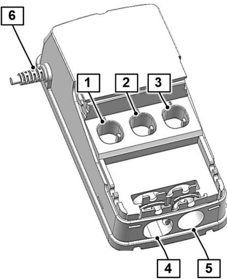
The diagram shows a perspective view of the CA 20 drive system. A power supply connector (6) is located on the left side. On the top surface, there are three circular ports labeled 1, 2, and 3. On the bottom surface, there are two circular ports labeled 4 and 5.
