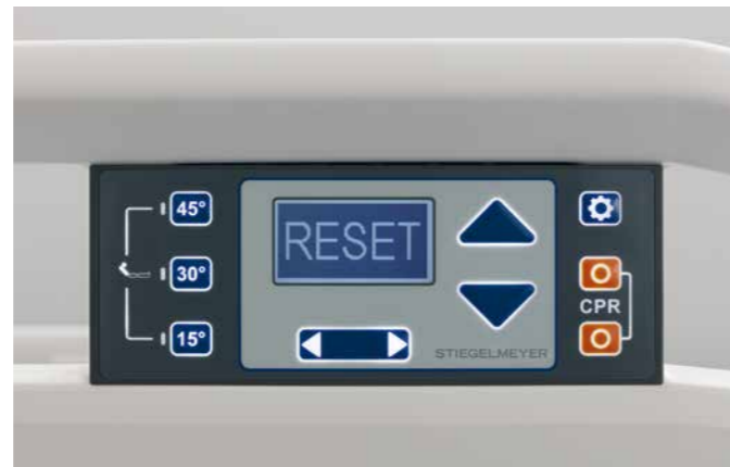
▲ The technician control level on the LCD handset and control panel provides useful settings for maintenance, error analysis and reset functions.
